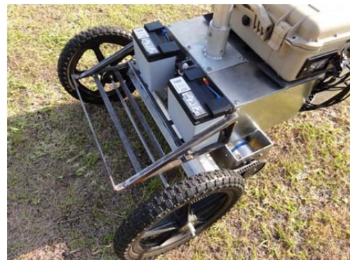
Figure 7: Lead acid batteries
